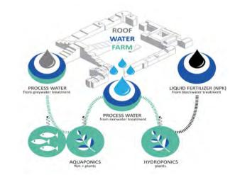
Figure 1: ROOF WATER-FARM Concept scheme. copyright: project ROOF WATER-FARM
